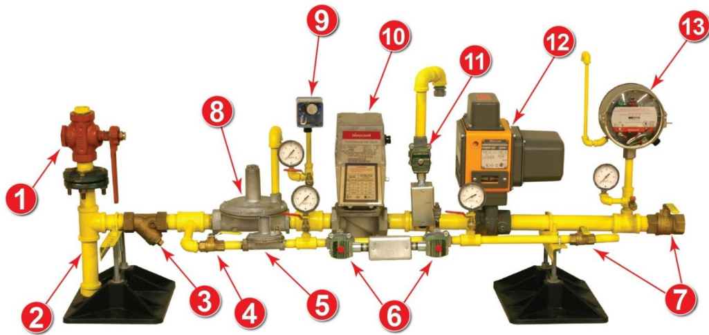
Note: Photo of Gas Train Simulator
