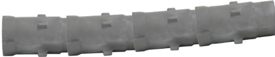
Figure 2: Self-recuperative burner inner tube
