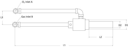
Figure 1: FHO96 Series Forehearth Oxygen Burner
