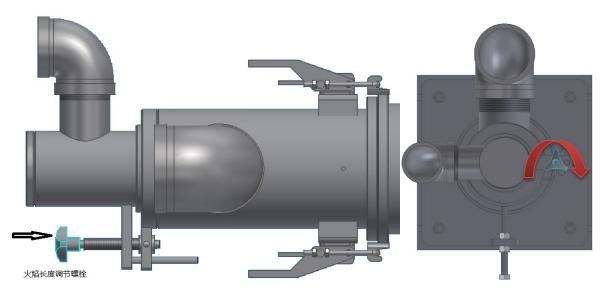
Figure 3: Diagram of FFO50 FlexFire® Oxygen Fuel burner adjustment knob
