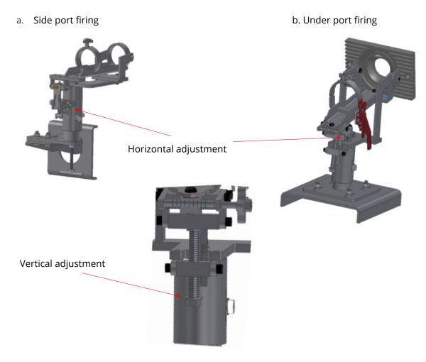
Figure 2. FlexFire® burner Adjustment Mechanism
