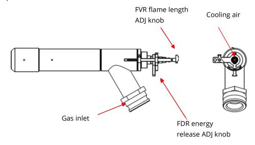
Figure 5: FlexFire® burner adjustment mechanism
