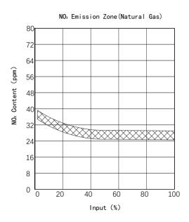
Fig 2. ANX70 Series Burner Operation Zone
