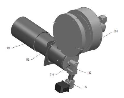
Fig 1. ANX70 Series Burner Explosion View
