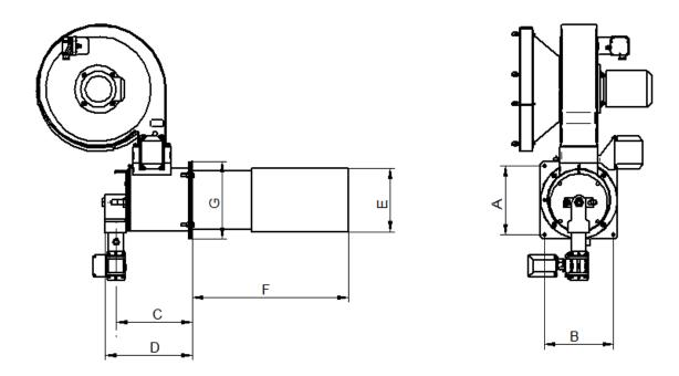
ANX70 Series burner installation dimension shown as table 2
