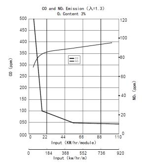
Fig 2. ANM77 Series Burner Operation Curve
