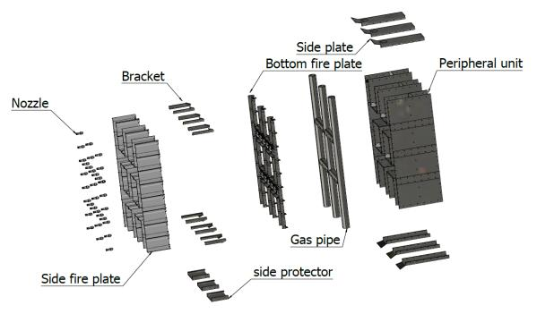
Fig 1. ANM77 Series Burner Explosion View
