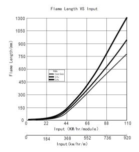
Fig 4. ANM77 Series Burner Input Curve Anderson Thermal Soluions (Suzhou) Co. Ltd.
