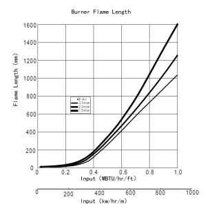
Fig 4. ANM75 Series Burner Input Curve
