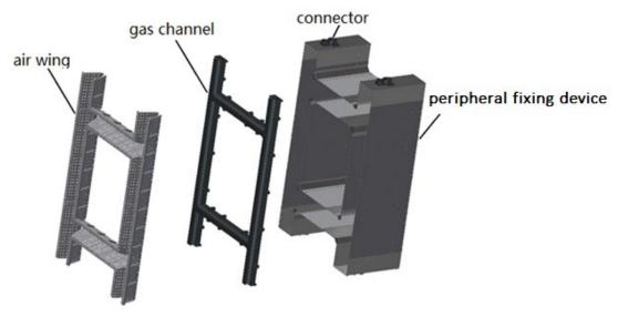
Fig 1. ANM75 Series Burner Explosion View
