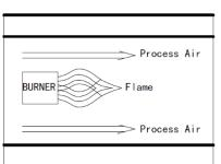
Parallel Process Flow -In Duct
